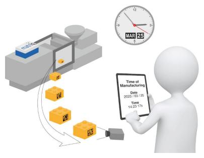
In parallel, the injection molding machine (IMM) stores data about the production cycle (called production protocol), including the cycle start time and cycle end time. The marked code is read by a code reader camera, to get the timestamp of that part. A database query is performed using the timestamp. The database returns the relevant cycle data for that part, helping to track when and how the part was produced.
